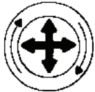
Rotate the filter while pulling straight out.
