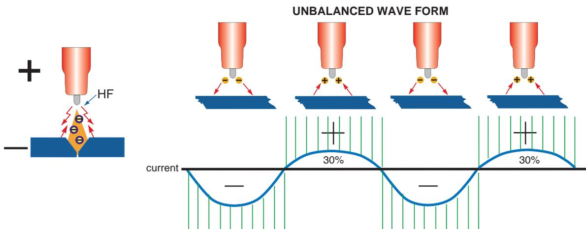
High-frequency voltage flows continually in the welding circuit and keeps the shielding arc in the welding area in an ionized state. When the arc is ionized the arc is maintained during the half of the cycle when the electrode is positive. However while the arc is maintained less current flows during this half of the AC cycle, producing an unbalanced wave.
