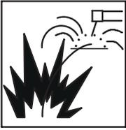
**Fire hazard.** Welding/cutting on closed containers, such as tanks, drums, or pipes, can cause them to explode. Flying sparks from the welding/cutting arc, hot workpiece, and hot equipment can cause fires and burns. Accidental contact of the electrode to metal objects can cause sparks, explosion, overheating, or fire. Check and be sure the area is safe before doing any welding/cutting.
