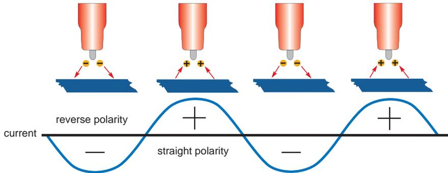
A square wave power supply can change the current from electrode + positive to electrode - negative very quickly. This produces high voltage as the current switches polarities allowing the arc to restart easily. The arc can be maintained without the use of high-frequency or any other arc stabilising methods.
