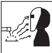
**Arc rays: harmful to people's eyes and skin.** Arc rays from the welding/cutting process produce intense visible and invisible ultraviolet and infrared rays that can burn eyes and skin.
