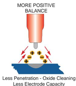
**Balance Adjusted for More Oxide Cleansing Action - Hotter Tungsten**
