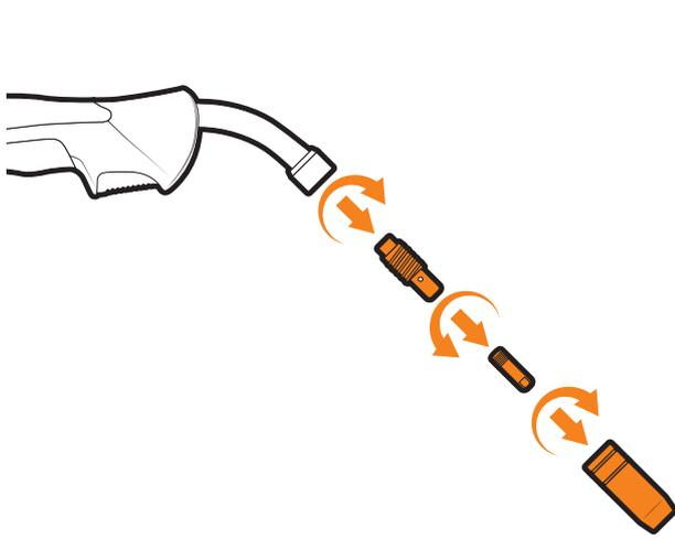
2 Remove the liner retaining nut.
