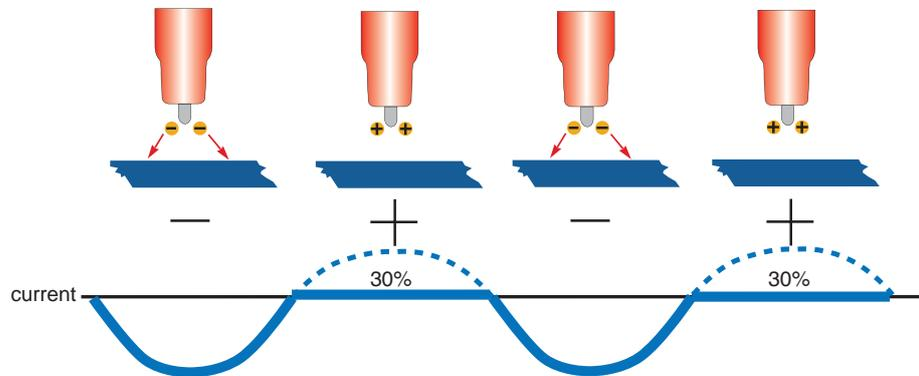
To overcome this lack of flow during one half of the cycle, a high-frequency (HF) voltage is generated and fed into the welding circuit. The HF maintains the arc stability during the half cycle when the electrode is positive.
