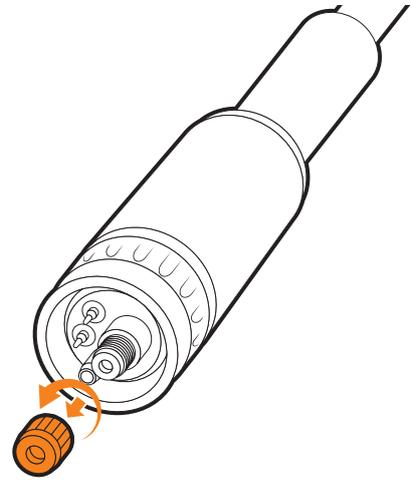
3 Carefully pull out and completely remove the existing liner. Ensure MIG torch is completely unraveled until setup is complete.
