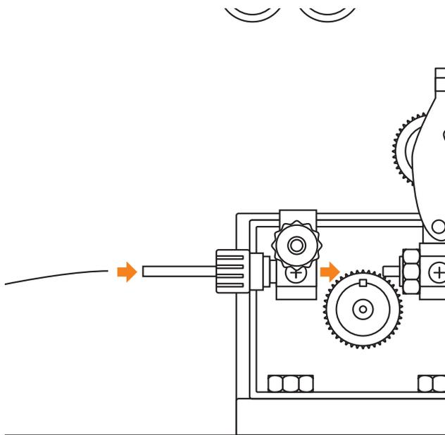
**12** Lift roller tension knob to lock wire in place. Twist to tighten.
