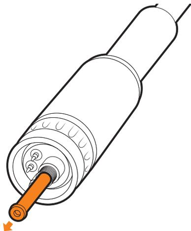
4 Fit the neck spring to the front end of the aluminium liner.
