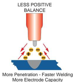
**Balance Adjusted for More Penetration - Cooler Tungsten**
