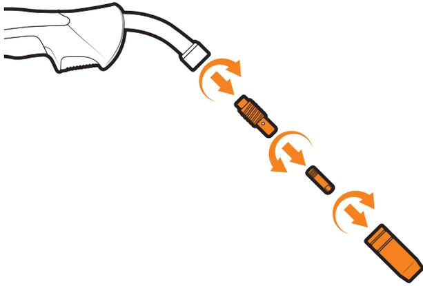
2 Remove the liner retaining nut.
