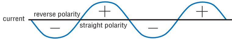
There are inherent problems that come with AC TIG arc rectification, arc stutter, arc wandering and arc stoppage. These problems typically occur during the transition between + and - cycles.
