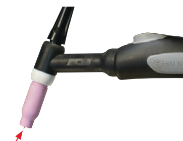
(1) Assemble the front end torch parts use the correct size and type of tungsten electrode for the job, the tungsten electrode requires a sharpened point for DC welding
