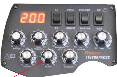
(12) Set the AC Balance knob between 4 & 5.
