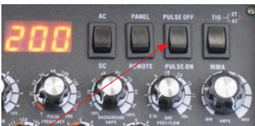
(6) Set the Pulse Selector switch to Pulse
