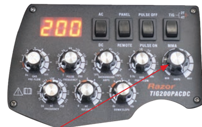
(3) Set the Peak Current (amps) to suit the tungsten size material type and thickness to be welded.
