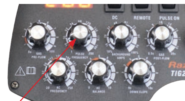
(4) Set the Pulse Frequency at 2 Hz
