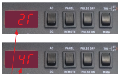
(2) Switch to the TIG function and the machine indicates what mode it is currently on (2T or 4T). To change the mode, switch off to MMA mode and back to TIG. Select 2T or 4T trigger function as required.
