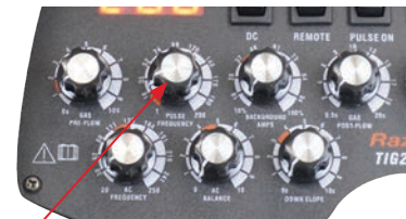
(4) Set the Pulse Frequency at 2 Hz
