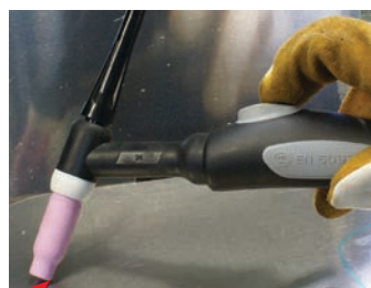
(13) Lay the outside edge of the Gas Cup on the work piece with the Tungsten Electrode 1- 3mm from the work piece
