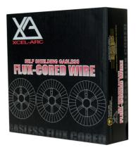
Xcel-Arc E71T-GS is an all-position, self-shielded flux-cored wire designed for single pass fillet and lap welding on galvanized or carbon steel as thin as 20 gauge, without burn-through. Gasless wire E71T-GS is commonly used on small portable 230 Volt welding machines, offering smooth arc action with very little spatter. Travel speed is fast, penetration is good and slag removal is easy.
