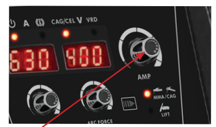
(7) Set the welding current using the amperage control dial
