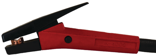
(8) Insert the Carbon between the jaws, the carbon should not extend too far out otherwise the air flow will not meet with the arc gouging zone at the workpiece.
