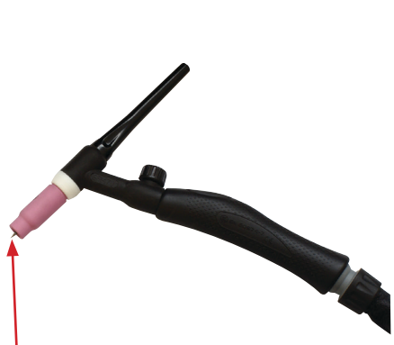
(5) Assemble front end parts of the TIG torch, fitting a sharpened tungsten suitable for DC welding.
