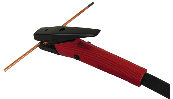
(9) Insert the Carbon between the jaws, the carbon should not extend too far out otherwise the air flow will not meet with the arc gouging zone at the workpiece.
