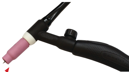
(8) Assemble front end parts of the TIG torch, fitting a sharpened tungsten suitable for DC welding.
