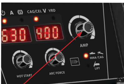
(3) Set the welding current using the amperage control dial
