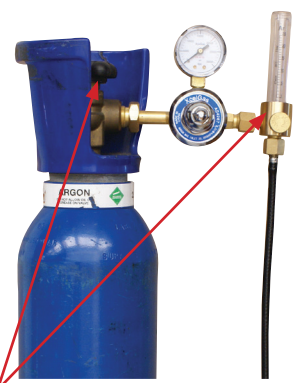
(6) Carefully open the valve of the gas cylinder, set the l/min to 6-12
