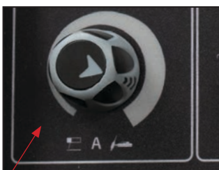
(4) Set the welding current using the amp control dial
