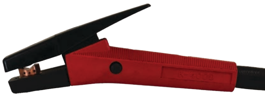
(9) Insert the Carbon between the jaws, the carbon should not extend too far out otherwise the air flow will not meet with the arc gouging zone at the workpiece.
