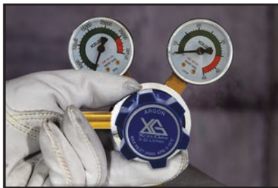
6) Carefully open the valve of the gas cylinder, set the Flow to 6-10 l/min.
