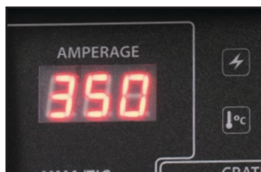
The set welding current will show on the digital amperage meter
