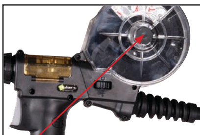
7) Push the cover release button to unlock the wire feed /spool cover.
