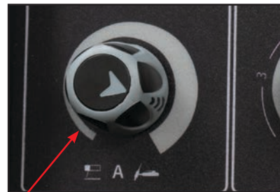
7) Set the welding current using the amperage control dial.
