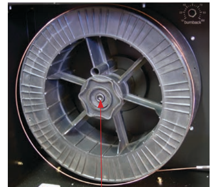
(8) The weight and speed of the wire spool turning creates an inertia that can cause the spool to run on and the wire loop over the side of the spool and tangle. If this happens increase the pressure on the tension spring inside the spool holder assembly using the tension adjustment screw.
