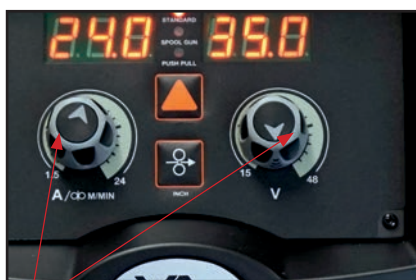
(15) Set welding parameters using the voltage and wire feed controls.
