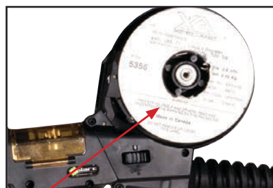
8) Place a spool of wire onto the Spool holder. Note: the spool retaining nut is Left Hand thread, turn it clockwise to undo it.
