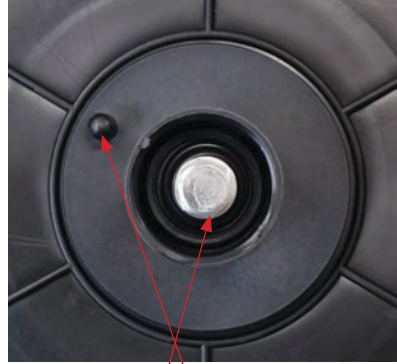
(2) Note the tension spring adjuster and spool locating pin.
