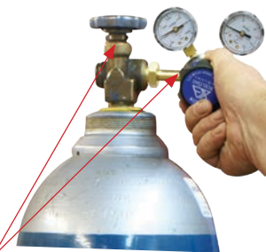
(14) Carefully open the valve of the gas cylinder, set the flow to 10 l/min
