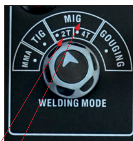
(16) Set the MIG function and desired trigger mode 2T or 4T.
