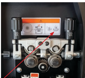
(16) Feed the wire through the drive rollers, apply light pressure on the drive rollers.
