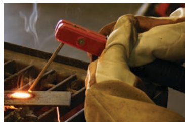
7) To finish the weld, break the arc by quickly snapping the electrode away from the work piece.
