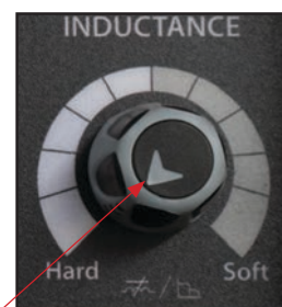
(17) Set the inductance with the front panel control knob. Less inductance for a tight hard arc, more inductance for a softer, wider arc.
