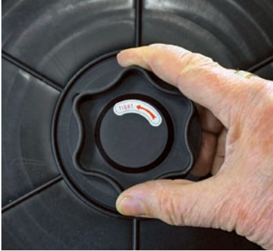
(1) Remove the spool retaining nut.
