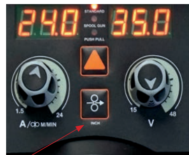
(11) Press and hold the inch wire button to feed the wire down the torch cable through to the torch head.
