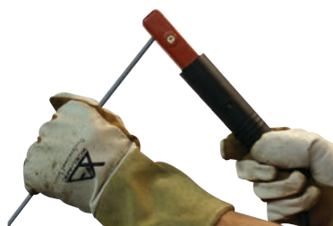
4) Place the electrode into the electrode holder and clamp tight.
