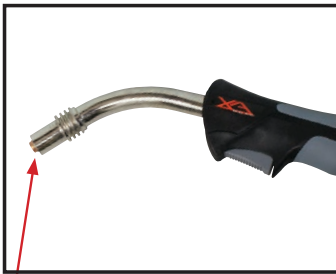
(1) Remove mig torch front end parts
