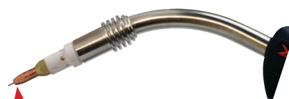
(17) Fit an Aluminium contact tip of the correct size to match the wire diameter being used
