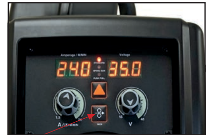
(11) Lay the torch cable straight or in a gentle curve on the floor. Use the inch button to feed the wire down the cable into the torch drive unit. Release the inch button when the wire reaches the torch drive unit.
