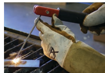
5) Strike the electrode against the work piece to create and arc and hold the electrode steady to maintain the arc
