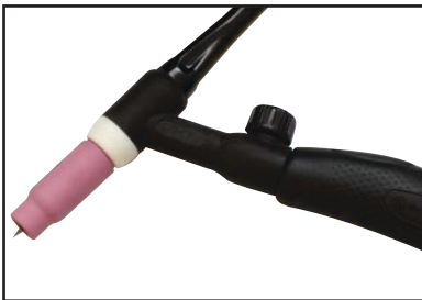
8) Assemble front end parts of the TIG torch, fitting a sharpened tungsten suitable for DC welding.
