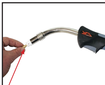
(8) Replace the front end parts
