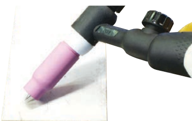
(7) To stop the welding, manually break the arc by with snappy lift away from the work piece.
