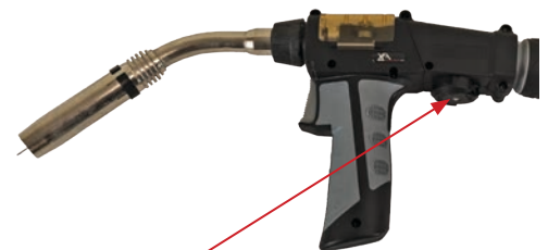
(17) Fine adjustment of the wire feed can be made remotely and during welding using the potentiometer located on the torch body
