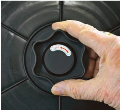
(1) Remove the spool retaining nut.
