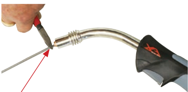
(7) Snip the liner off 3mm past the end of the torch neck.
