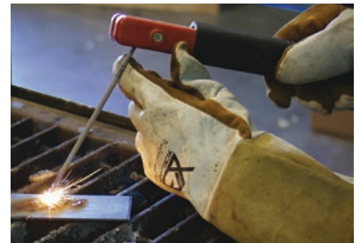
5) Strike the electrode against the work piece to create an arc and hold the electrode steady to maintain the arc
