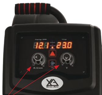
(16) Set welding parameters using the voltage and wire feed controls.
