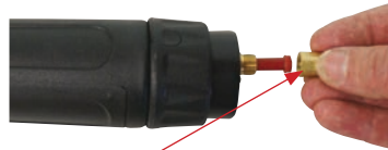
(2) Remove the liner retaining nut
