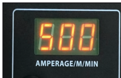
The set welding current will show on the digital amperage meter
