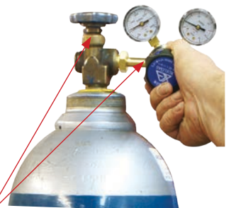
(14) Carefully open the valve of the gas cylinder, set the flow to 10 l/min
