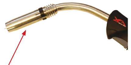
(18) Fit the remaining front end parts to the torch neck ready for welding.
