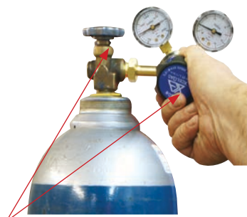
(15) Carefully open the valve of the gas cylinder, set the flow to 12-18 l/min
