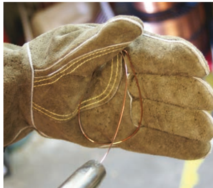
(8) A simple check for the correct drive tension is to bend the end of the wire over hold it about 100mm from your hand and let it run into your hand, it should coil round in your hand without stopping and slipping at the drive rollers, increase the tension if it slips.
