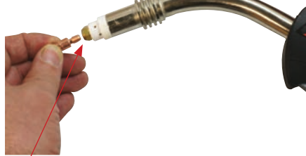
(10) Remove the gas nozzle and contact tip from the front end of the mig torch.
