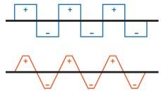
**AC Square Wave:** Allows the current to change from electrode + positive to electrode - negative very quickly. This produces high voltage as the current switches polarities allowing the arc to restart easily. The arc can be maintained without the use of high-frequency and the fast transitions provide for responsive, dynamic and focused arc for better directional control.
