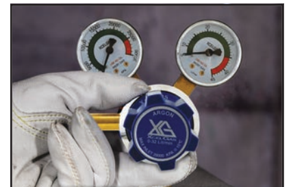
14) Carefully open the valve of the gas cylinder, set the flow to 6-10 l/min
