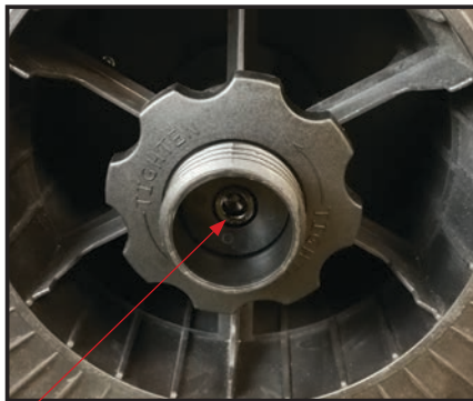
(8) The weight and speed of the wire spool turning creates an inertia that can cause the spool to run on and the wire loop over the side of the spool and tangle. if this happens increase the pressure on the tension spring inside the spool holder assembly using the tension adjustment screw. NOTE: As wire volume reduces spool brake tension may also require re-adjustment
