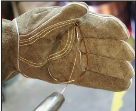
(9) A simple check for the correct drive tension is to bend the end of the wire over hold it about 100mm from your hand and let it run into your hand, it should coil round in your hand without stopping and slipping at the drive rollers, increase the tension if it slips.
