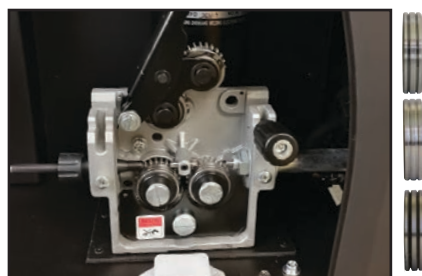
6) Fit the correct type and size of drive rollers.V Groove for Hard Wires. U Groove for Aluminium. Knurled for Flux Cored
