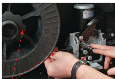
(7) Place wire onto spool holder. Feed the wire through the inlet guide tube into the drive roller.
