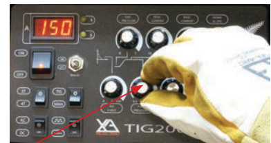
(4) Set the Pulse Frequency at 2 Hz
