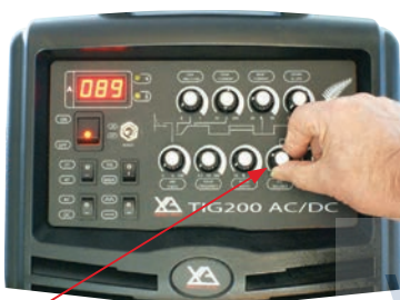
(12) Set the AC Balance Control to 25%
