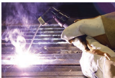
6) Hold the electrode slightly above the work piece to maintain the arc while travelling at an even speed to create an even weld deposition.
