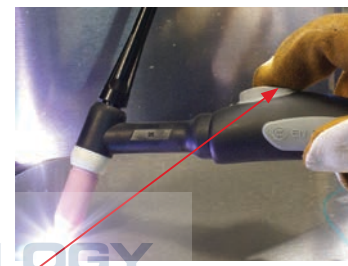
(14) Press the torch switch and the arc will ignite across the gap between the tungsten and work piece. Hold even distance of about 2mm gap between the tungsten and work piece to maintain the arc.
