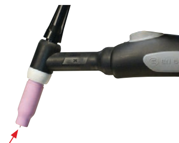
(9) Assemble the front end torch parts use the correct size and type of tungsten electrode for the job, the tungsten electrode does not require a sharpened point for AC welding
