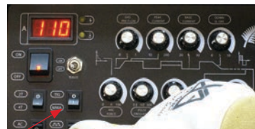
(6) Set the Pulse Selector switch to Pulse
