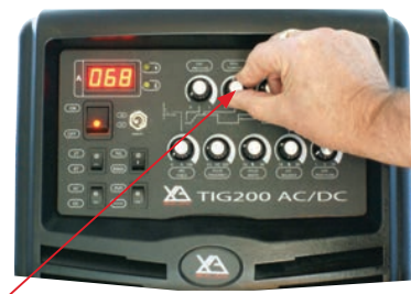
(3) Set the Peak Current (amps) to suit the tungsten size material type and thickness to be welded.
