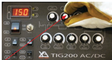
(2) Set the Peak Current at 110 Amps
