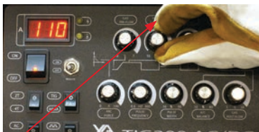
(2) Set the Peak Current at 110 Amps
