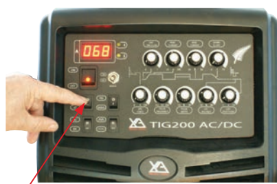
(2) Select 2T or 4T trigger function as required
