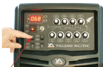
(10) Select 2T or 4T trigger function as required
