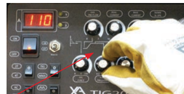
(4) Set the Pulse Frequency at 2 Hz
