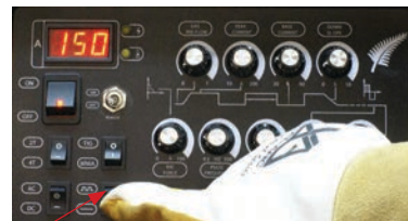
(6) Set the Pulse Selector switch to Pulse
