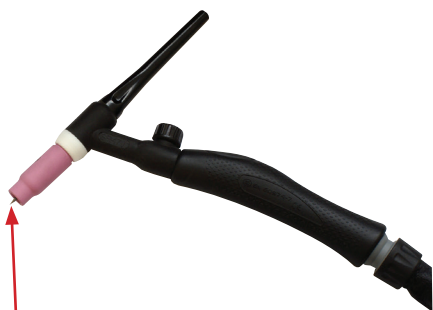
(5) Assemble front end parts of the TIG torch, fitting a sharpened tungsten suitable for DC welding.
