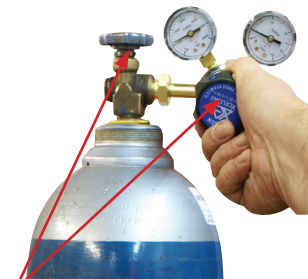
(15) Carefully open the valve of the gas cylinder, set the flow to 6-10 l/min
