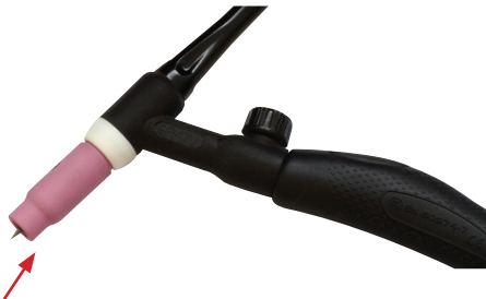
(5) Assemble front end parts of the TIG torch, fitting a sharpened tungsten suitable for DC welding.
