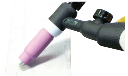
(7) Lay the outside edge of the Gas Cup on the work piece with the Tungsten Electrode 1- 2mm from the work piece.
