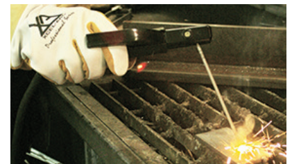
5) Strike the electrode against the work piece to create an arc and hold the electrode steady to maintain the arc
