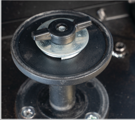
(1) Remove the spool retaining nut.
