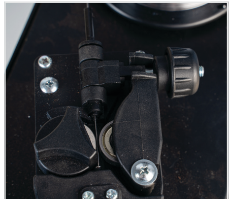
(6) Lock down the top pressure roller and apply a medium amount of pressure using the tension adjustment knob
