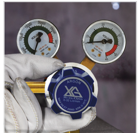
(12) Carefully open the valve of the gas cylinder, set the flow to 8-10 L/min
