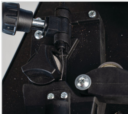
(5) Feed the wire through the drive roller and into the outlet guide tube of the wire feeder.
