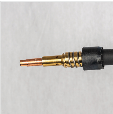
(10) Fit the correct size contact tip over the wire and fasten tightly into the tip holder.
